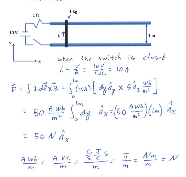
(12 pts) 10. One thing we have ignored with the rail system in problem 9 is that as the bar accelerates, there will be a changing flux in the circuit. This will result in an Vemf that will oppose the 10V, reducing the current and reducing the force on the bar. When Vemf = 10 V the force will have gone to aero on the bar. So the bar will have reached a maximum velocity. What is this maximum velocity for the rail system of problem 9?
